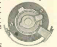
Floating contact shoe glides over resistance element in
