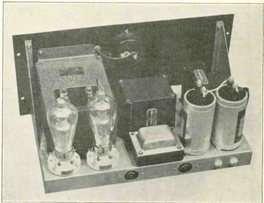
The lower section of the relay rack holds most of the power supply equipment, as shown above. The low-voltage power transformer, high-voltage power transformer, two 2 mfd. 2000 volt Aeovox oil-filled transmitting condensers, rectifier filament transformer, two 866A rectifier tubes, heavy duty choke for the high-voltage filter and the milliammeter are clearly shown.
